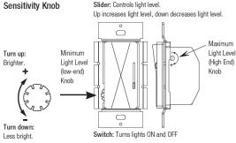
IMPORTANT: To avoid lights turn off or flicker at low end: Push slide down. Turn the low-end knob clockwise until the lights remain on without flickering.
